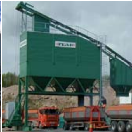
3 compartment square silo and inclined skip track
